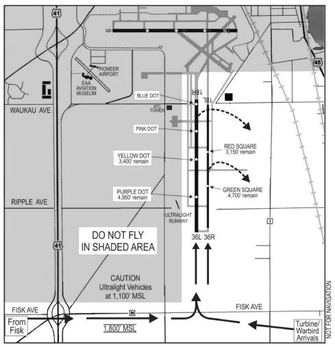
If a go-around is needed, notify ATC immediately and do not continue past ATC Tower. If unable to notify ATC, make a right turn to the southeast prior to ATC tower for resequencing.
