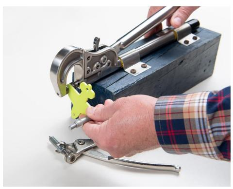
**Step 7** – Remove the final cleco, insert and squeeze a third rivet on the opposite wing tip.
