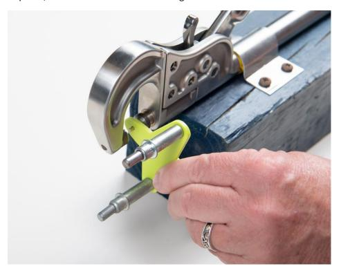
Step 5 – Fully squeeze the rivet by pressing downward on the rivet squeezer handle to "set the rivet".
