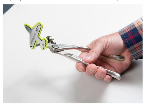
**Step 3b.** – Insert a second cleco at the opposite wing tip to properly align the holes at the nose of the airplane key chain.
