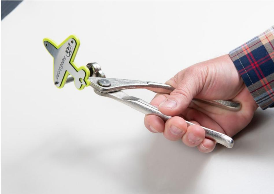
**Step 3b.** – Insert a second cleco at the opposite wing tip to properly align the holes at the nose of the airplane key chain.
