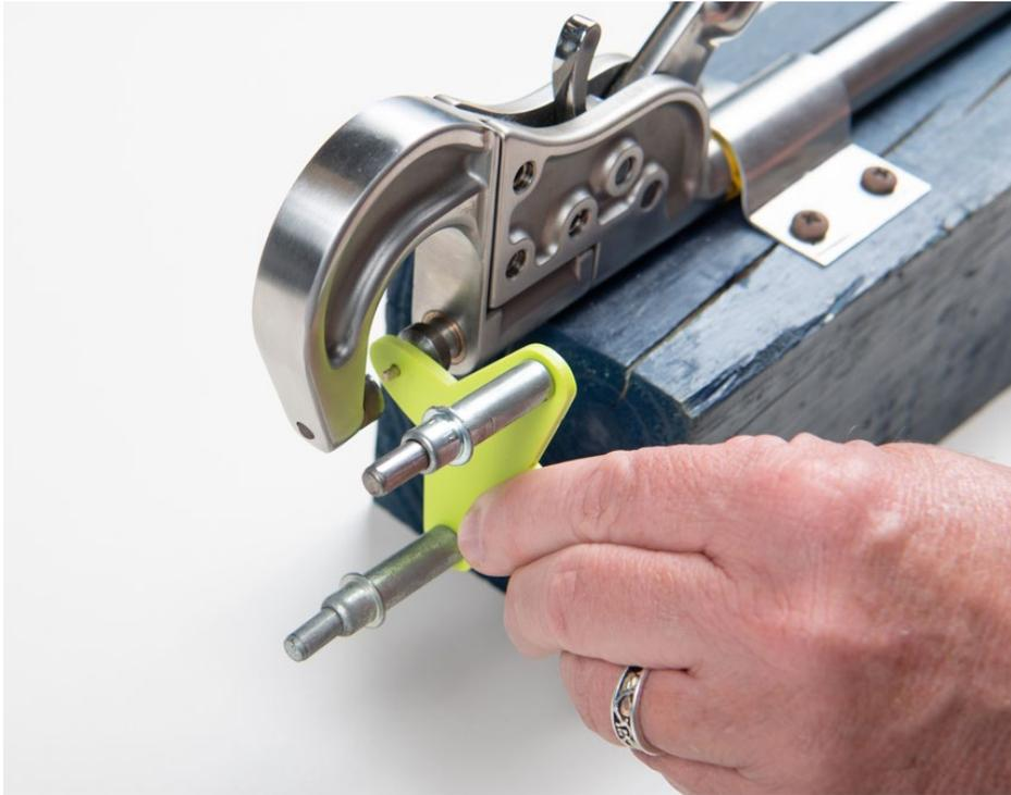
**Step 5** – Fully squeeze the rivet by pressing downward on the rivet squeezer handle to “set the rivet”.
