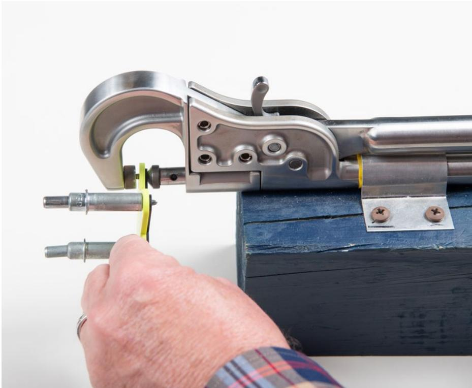
The free end of the rivet will deform to a mushroom shape to permanently secure the assembly.
