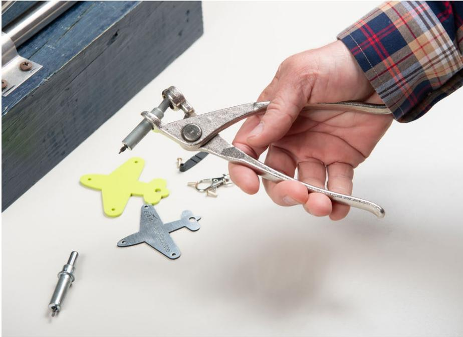
**Step 2** – Squeeze the cleco pliers to enable the cleco to fit into the holes of the key chain parts.
