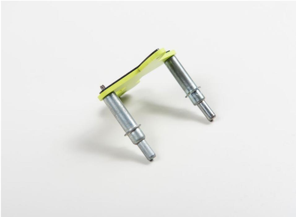
**Step 4** – Insert a rivet from the top surface of the key chain through the hole at the nose of the airplane, then set the head of the rivet against the rivet set as shown.
