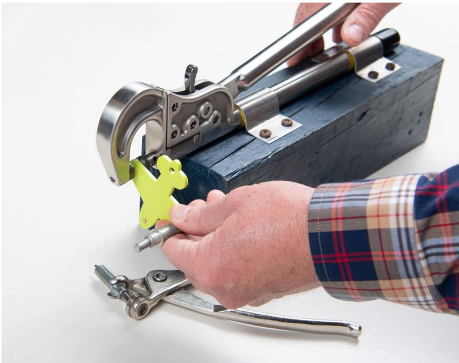
**Step 7** – Remove the final cleco, insert and squeeze a third rivet on the opposite wing tip.
