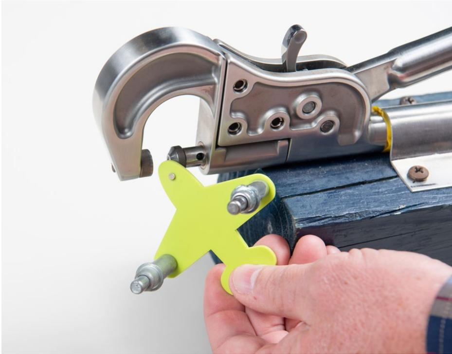
**Step 6** – Using the cleco pliers, remove one of the two clecos, then insert a second rivet and set the rivet firmly in place.
