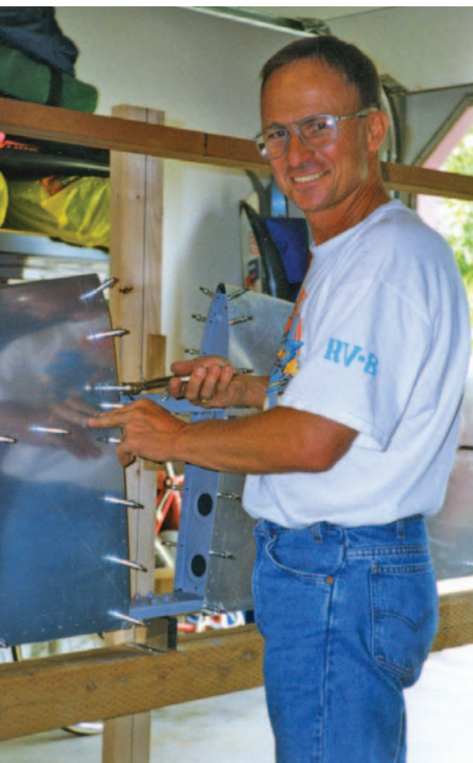
Lauran Paine is all smiles as he Clecos the fuselage sides together in preparation for riveting the all-metal airplane.
